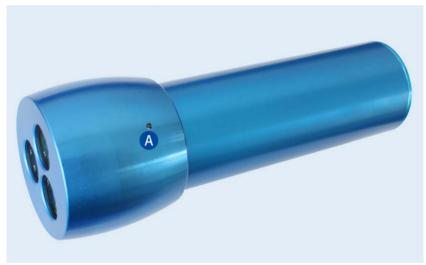
2. Draw the housing parts apart carefully to remove the batteries from the grip.
