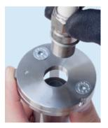
3 The integrated quickrelease lock guarantees rapid changes and secure holding of the spark plugs while they are being set.
