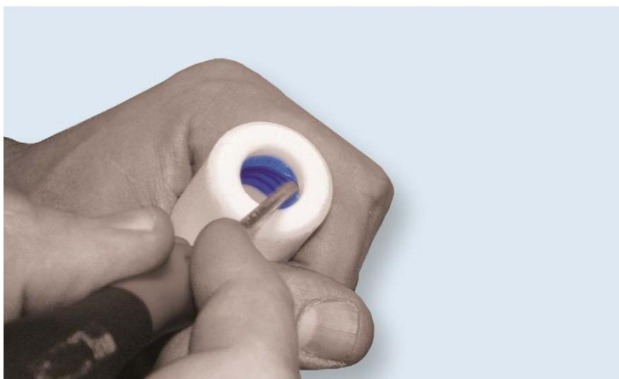
5. Position the silicone seal with the screw driver accurately along the slot and check fit. The seal must flush with the bore of the teflon extension.
