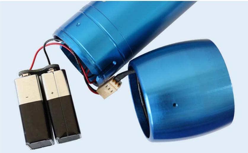
3. Carefully detach the empty batteries from the connection clip and insert two new 9-volt batteries.
